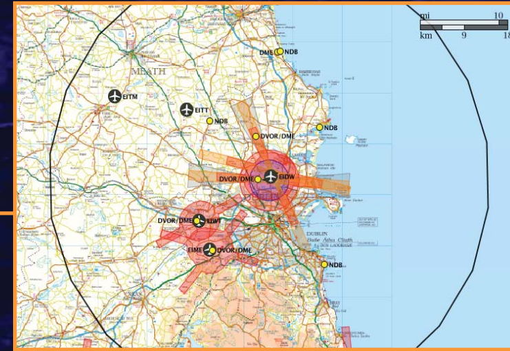
Area 3 (Aerodrome Area): Map of Dublin International with various obstacles marked by orange triangles and obstacle limitation surfaces shown.
